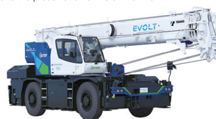
Electric rough terrain crane EVOLT eGR-250N
