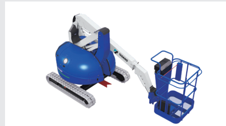
NUL07E-7, electric crawler type articulated boom aerial work platform
