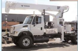
The new TM-20110 boom truck (above) has a maximum tip height of 120 feet. Like the established TM-1882 (left), it has the longest boom in its class.
