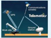
The new Hello-Net crane management system from Tadano enables crane owners to remotely monitor the operating parameters of their machines from anywhere in the world by internet.
