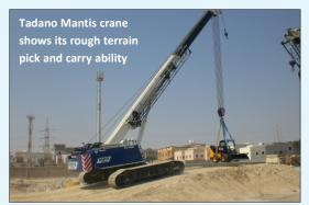
A GTC-400EX and a GTC-700EX were each put through their paces, demonstrating their ability to pick and carry their full load capacity through 360 degrees, to boom up and out with full load, to climb steep gradients, and to counter rotate on the spot.
