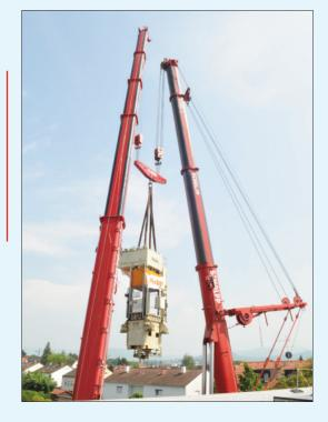
transport costs. The ATF 400G-6 can lift loads that other cranes this size cannot lift and is compact enough to work on sites that other cranes with its capacities cannot get onto.
