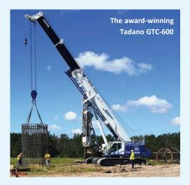
Series. The design project was managed by Tadano Mantis and included collaboration with Tadano Ltd in developing the purpose-designed, Tadano-built telescopic boom and the integration of Tadano winches, jib, hydraulic cylinders, AML-C rated capacity indicator and Hello-Net telematics.
