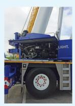
The engine of the new ATF 60G-3 is mounted to the rear of the rotating upper works, and not just behind the driver's cab
