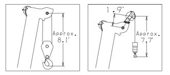
NOTE:1.Boom geometry shown is for unloaded condition and machine standing level on firm supporting surface. Boom deflection and subsequent radius and boom angle change must be accounted for when applying load to hook.
