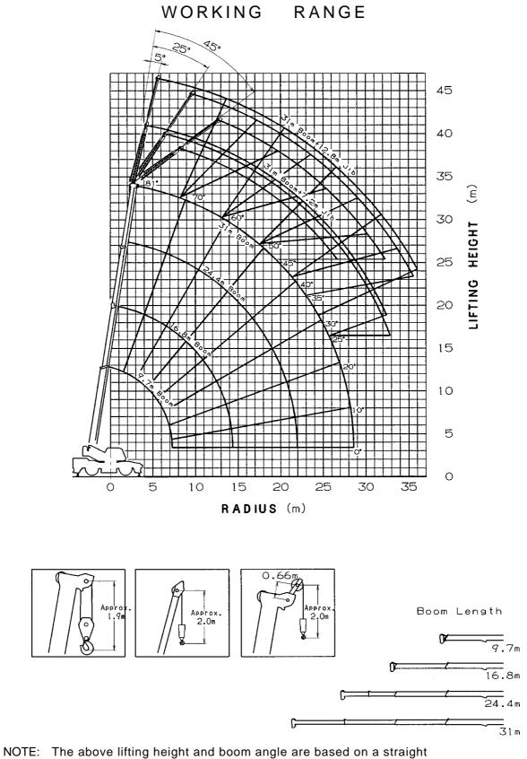
(unladen) boom, and allowance should be made for boom deflection obtained under laden conditions. The above working range is shown on condition with outriggers fully(6.3m) extended. DIMENSIONS
