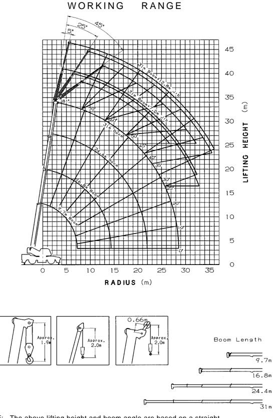
NOTE: The above lifting height and boom angle are based on a straight (unladen) boom, and allowance should be made for boom deflection obtained under laden conditions. The above working range is shown on condition with outriggers fully(6.3m) extended. DIMENSIONS
