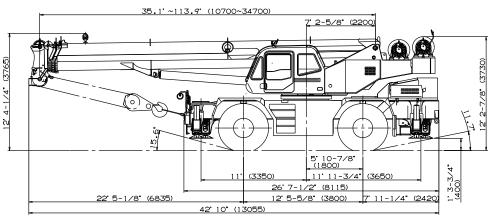
Note : Dimension is with boom angle at -0.8 degree. ( )Reference dimensions in feet
