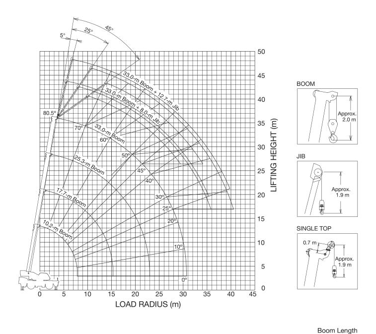
NOTE: Boom and jib geometry shown are for unloaded condition and machine standing level on firm supporting surface.
