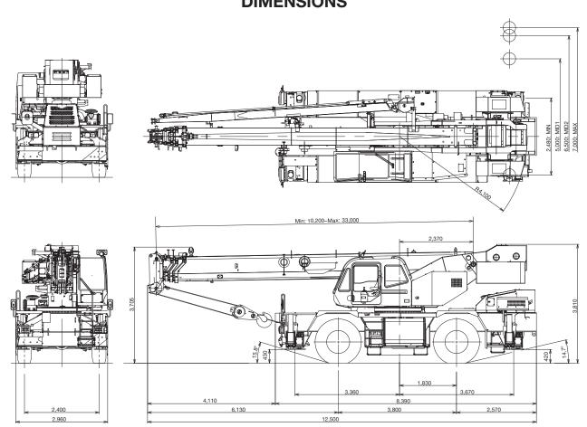
Note: Dimension is with boom angle at -1 degree.
