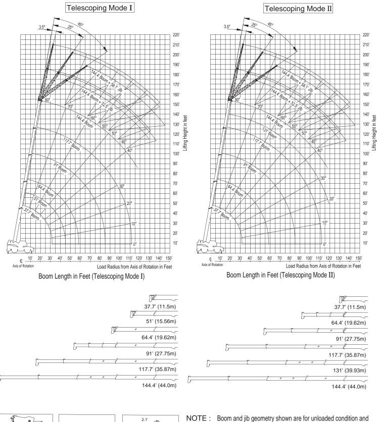
DTE : Boom and jib geometry shown are for unloaded condition and machine standing level on firm supporting surface.
