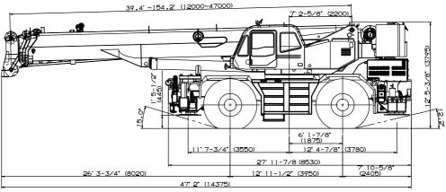
Note: Dimension is with boom angle at -1.5 degree.
