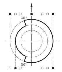
Front jack not extended FL outrigger extended to fully, FR outrigger extended to minimum RL outrigger extended to minimum
