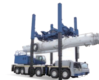
All Terrain Crane Mounting / Removal Lifter (Example of boom removal from ATF400G-6)
