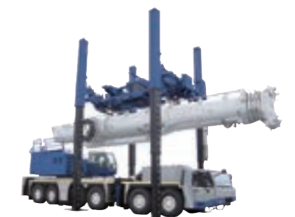
All Terrain Crane Mounting / Removal Lifter (Example of boom removal from ATF400G-6)
