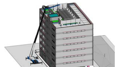
Illustrative image with Tadano crane data incorporated in a BIM Model
