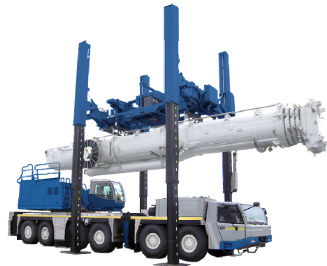
Example of boom removal from All Terrain Crane, ATF400G CL-500 (Released on August 2013)
